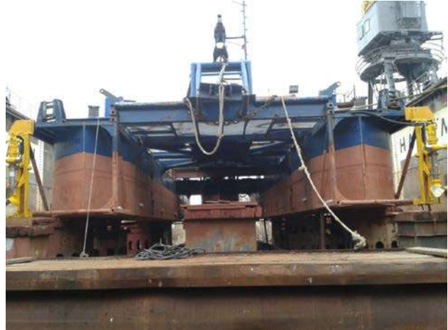
The Trimaran Rossana assembly at CMC dry-dock
