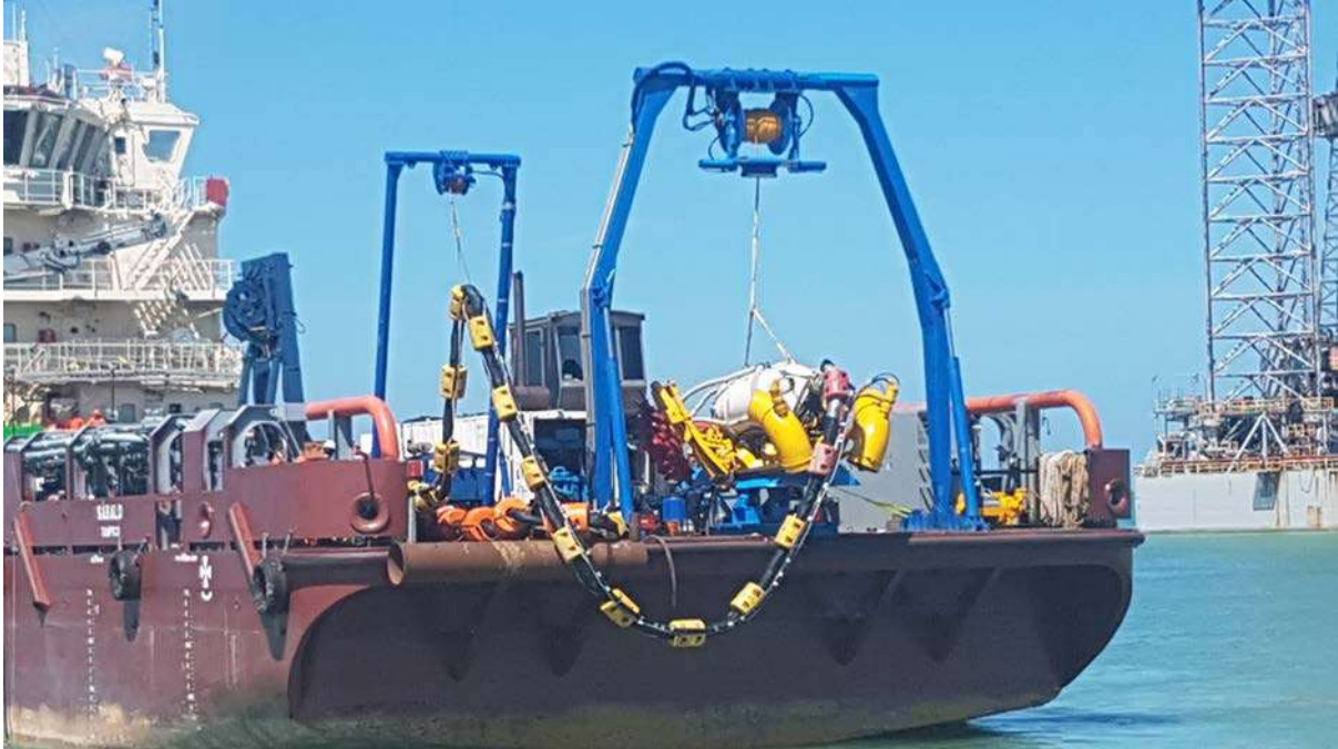
TSV SABALO equipped with L.A.R.S. and trenching spread.
